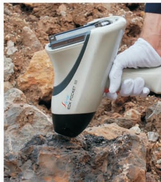
● There is a wide range of samples in the geographic and mineral industries: rocks, soil, sediment, ores, etc. They have complicated compositions and require rapid and accurate qualitative and quantitative analysis on the site or in the field. Besides, if tests are to be carried out before large-scale production, they must produce results as quickly as possible. Therefore, two features are ascribed to this industry: sample complexity and measurement rapidness.
